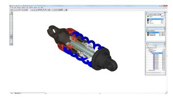
Manipulate 3D data to create a cutaway that depicts either a precise part or several components.
